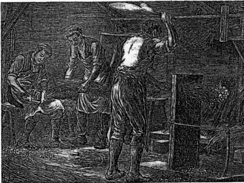
Figure 4. The men on the left are preparing the dried flax plants for seed removal. The man in the center is beating the seeds off the stalk by holding the stems over a scutching board and striking them with a scutching knife. Once removed, the seeds fall to the floor onto a winnowing cloth that facilitates easy collection. “Hand Scutchers at Work,” from Great Industries of Great Britain , vol. 1 (London: 1877–1880?), 212. Permission of the American Textile History Museum, Lowell, Massachusetts.
